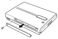
**3** Extract the tape from the inside of the unit with an elongated object, as illustrated.
